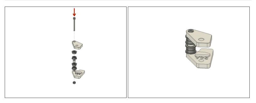
Assemble pulley brackets
