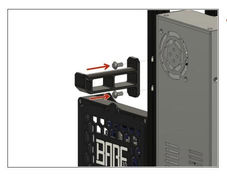
Attach Spool Holder with M5x10 screws and M5 drop-in T-nuts
