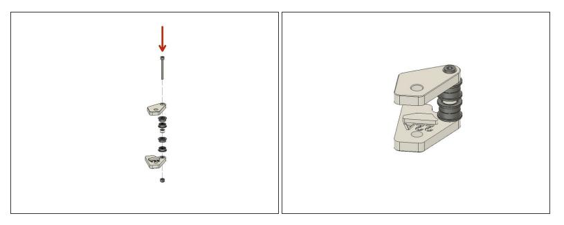
Assemble pulley brackets
