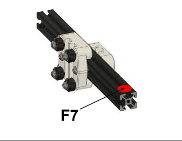
Attach Z carriage and leadnut assembly to F7 using M5x45 screws and M5 Nylock nuts
